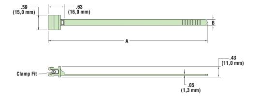
MaterialNylon 6/6 UV Resistant and Heat StabilizedFlammability Rating94V-2Temperature Range-.04°F (-18°C) to 221°F (105°C)
